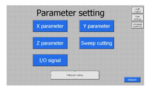
Click the 5 parameter setting in the parameter setting to enter the respective setting screen. The cutting mode button switches respectively: horizontal push test cutting, sweep cutting and chop cutting;
